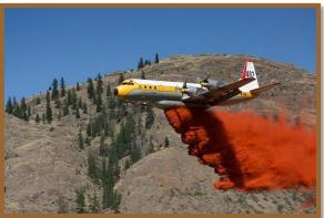
They contain ammonium salts which affect the burning process of forest fuels. Retardants prematurely release the gaseous fuels within logs and debris. This reaction releases a water and carbon dioxide combination that cools and suffocates the fire. Retardant has a much longer-lasting effect than water in fire suppression because it does not evaporate.
